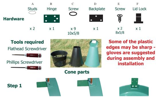
Place the ribbed side of the hinge on the inside of the lid. Screw the hinge (B) on to the lid through the pre-drilled holes using the two studs (A). Do not over tighten the studs as you could crack the lid.
